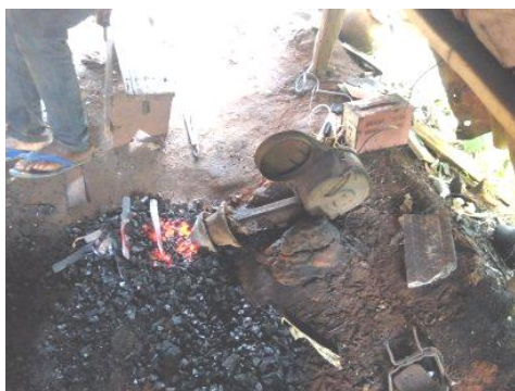
Plate 3: Electric Motor Propeller with to Tuyere Nozzle (Anyaku and Eko Uzu)
