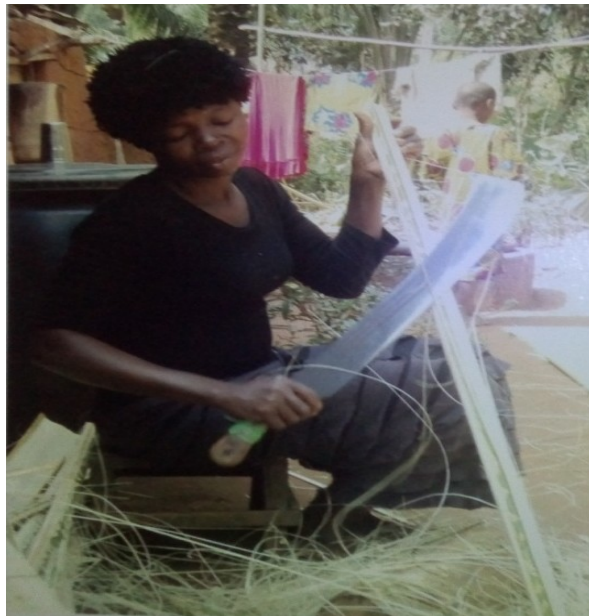
Plate 3: Processing of ekwele fibre from the leaf stalk of African oil palm.
