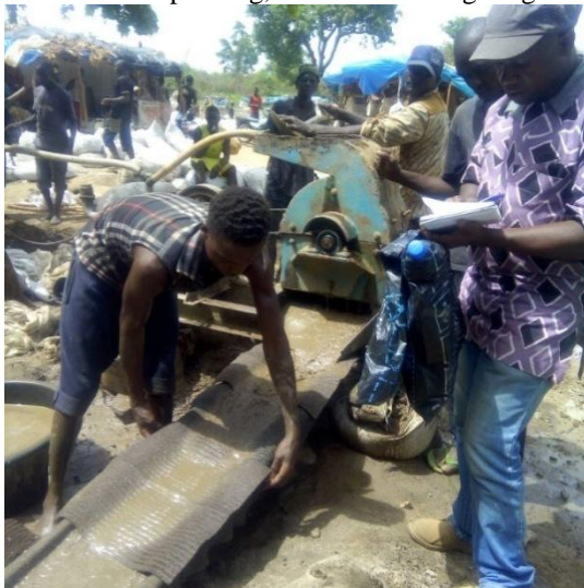
Plate 4 (a) Milling and Sluicing of Ore
