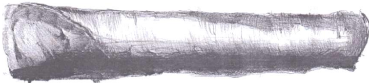
Fig.6 Chizu (Local made chisel): Used for cutting some part of metal before sending it to the furnace Drawing by Nzoiwu, Azuka 2018
